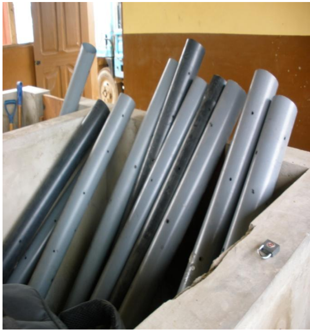
Aeration pipes to be inserted into composting organic matter
